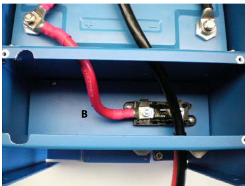
24V battery – single cable For CB battery type place 1x link #B. For BMS battery type make BMS cables connections first before placing this link!
